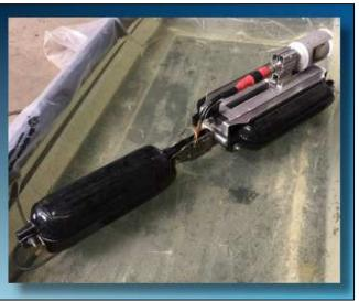
The hinged design worked well to allow for easy manoeuvring and insertion into drain lines from catch basins. Next, a cage was required to protect the camera from the top of the pipe if the water level was particularly high. Trent decided that a welded aluminum cage would provide protection, be light weight, look good, and be a strong point for lowering the raft into a drainage system.
