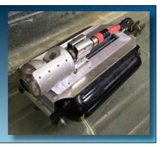
The next stage was to deal with the tether. Because the camera would be pulling against the tether, and the weight of the tether would be affecting the stability and balance of the system, a solution was required. This answer was a separate raft, hinged and balanced, to carry the weight of the cable and absorb any tether pull in unwanted directions.
