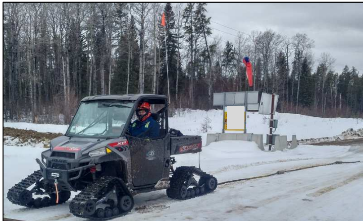
FIGURE 1: ATV used to transport GPR system with GPR antenna in tow
