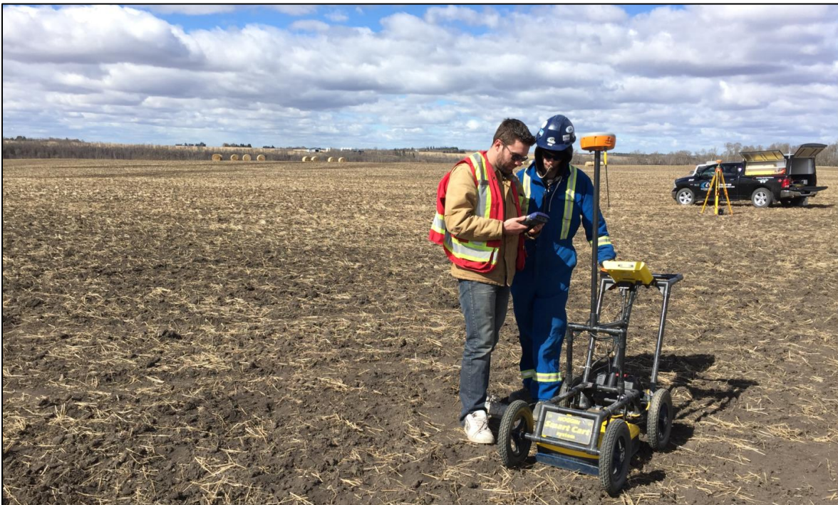
Figure 3: Howard Black and Matt Etherington configure the RTK GPS to one of Maverick's GPR systems to provide positional data. The wavelength of radar system, deployment platform, and data gathering method was chosen based on the site and suspected targets.
