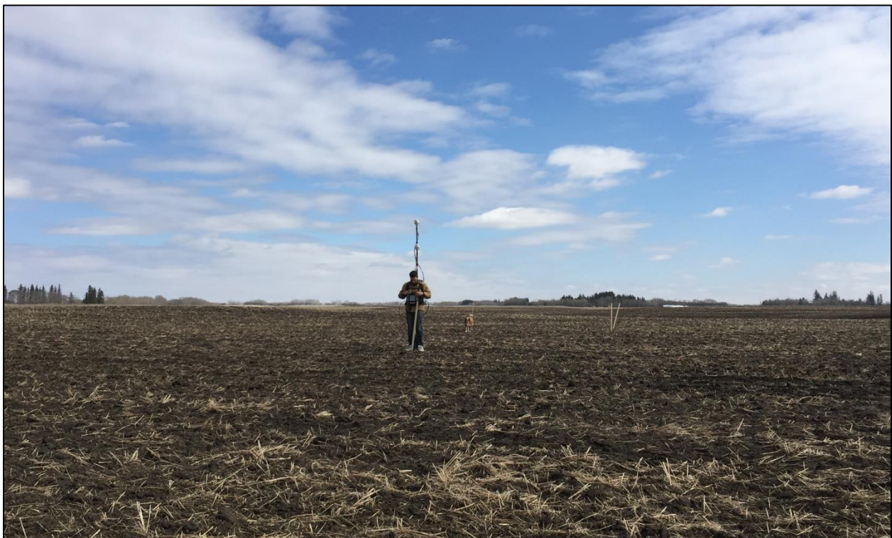
Figure 6: Howard Black collecting Mag data in the open field. Magnetic Gradiometry data can be gathered and analyzed relatively quickly, however real-time interpretations are limited and metallic objects or debris can have a negative effect on the results.
