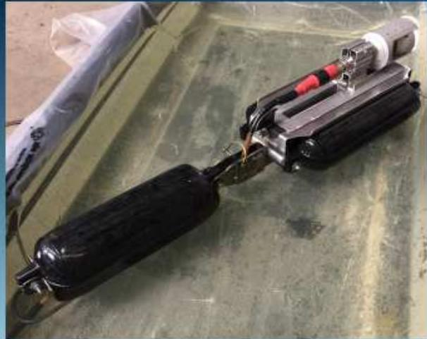
The hinged design worked well to allow for easy manoeuvring and insertion into drain lines from catch basins. Next, a cage was required to protect the camera from the top of the pipe if the water level was particularly high. Trent decided that a welded aluminum cage would provide protection, be light weight, look good, and be a strong point for lowering the raft into a drainage system.
