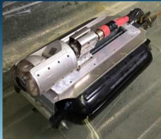
The next stage was to deal with the tether. Because the camera would be pulling against the tether, and the weight of the tether would be affecting the stability and balance of the system, a solution was required. This answer was a separate raft, hinged and balanced, to carry the weight of the cable and absorb any tether pull in unwanted directions.
