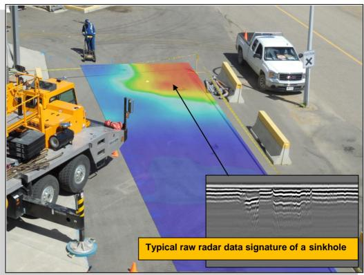
How do we look for underground hazards? Maverick regularly performs Ground-penetrating Radar (GPR) on sites to gather data for coordinators and engineers to evaluate subsurface conditions prior to setting up for critical crane lifts, as well as ice roads, pipeline crossings, bridge components, structural slabs, and other radar applications - helps us trust the ground we walk and work on.
