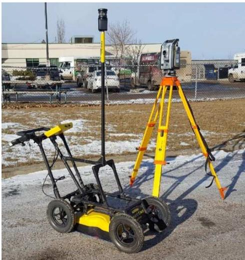
**THE SOLUTION:** A series of Ground Penetration Radar (GPR) scans were conducted over the course of several weeks, as areas became available. The systems that Maverick Inspection Ltd. utilized on this project are the Noggin250® and the Noggin500® made by Sensors & Software Inc.
