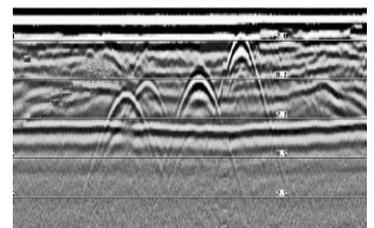
The GPR software employed by Maverick is able to provide quantitative results with regards to depth of coverage, concrete thickness, rebar spacing and other often unknown information. This quantitative information can then be used with CAD programs to build 3D models in a computer showing a very clear representation of subsurface features.
