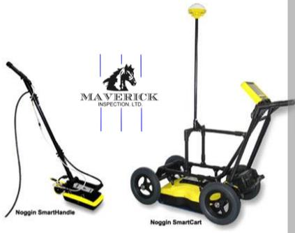
*How do we look for underground hazards? Maverick regularly performs Ground-penetrating Radar (GPR) on sites to gather data for coordinators and engineers to evaluate subsurface conditions prior to setting up for critical crane lifts. This work - and similar data gathering for ice roads, pipeline crossings, bridge components, structural slabs, and other radar applications - helps us trust the ground we walk and work on.*
