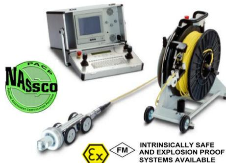
The T66 crawler & camera system is small and robust with pan and tilt features for pipelines as small as 4" up to 30" diameter. The T66 can travel over 660' and can maneuver around 45°/90° elbows. The system is equipped with a built in ATC (Automatic Tilt Compensation). The EX rating of the crawler is ideal for hazardous environments, such as work in the oil & gas industry.
